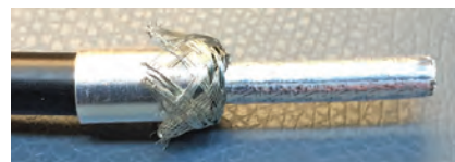
Figure 4 — The cable braid shown trimmed and folded back.
