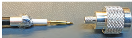
Figure 6 — The center pin being fitted.
